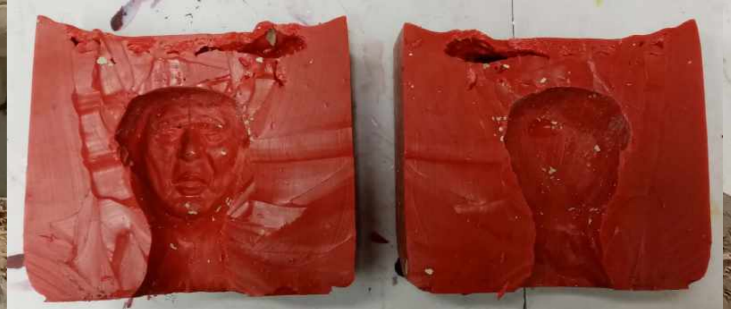
STEP 3 - REMOVE THE WALLS AND CUT THE MOULD IN HALF...
